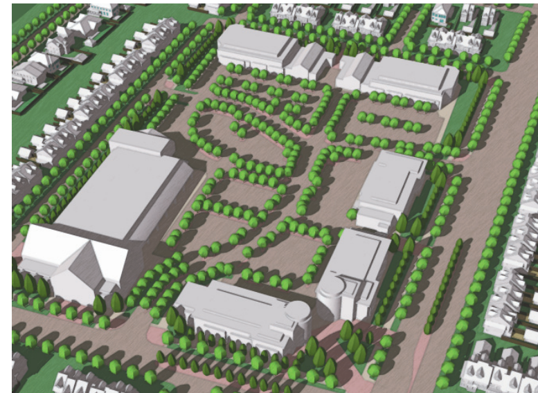
Figure 47: Create connections between buildings and subdivide interior parking areas with planted drive aisles and walkways.
