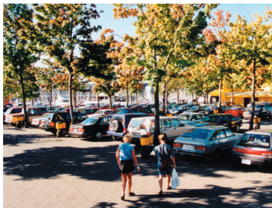
Photo 28: This parking lot on Granville Island features porous pavers and trees that provide shading, preventing the Heat Island Effect.
