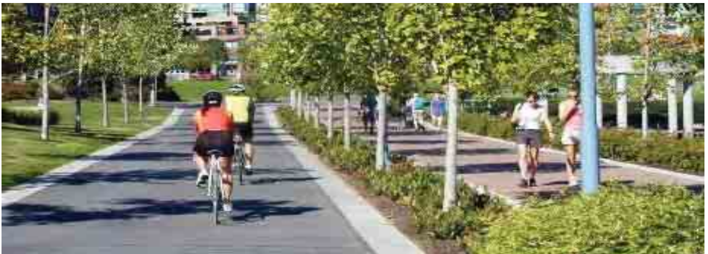
Multi-use paths should reflect their function, and where necessary, clearly differentiate between walking and cycling routes.
