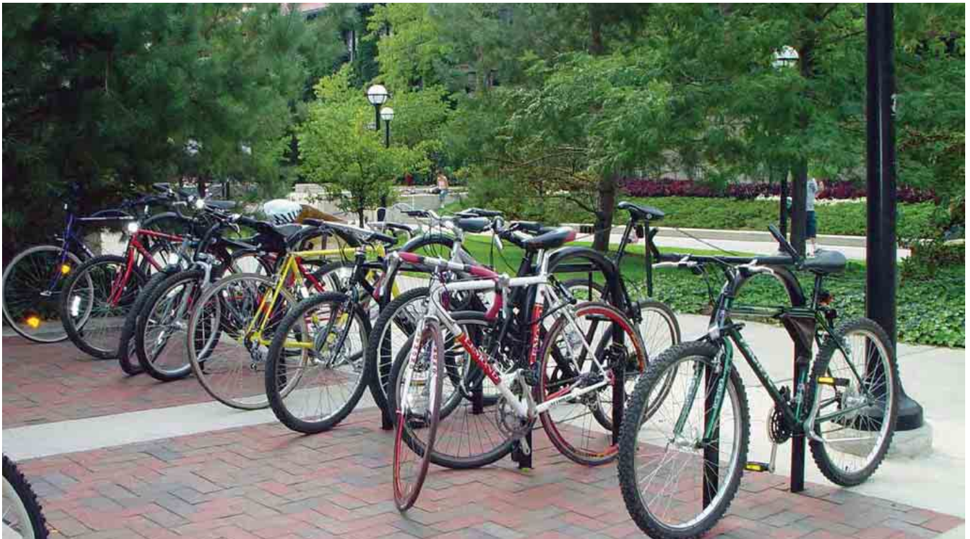
Bicycle parking should be conveniently located within areas of high pedestrian activity, such as Neighbourhood Centres and nodes. A simple post-and-ring, or similar style is recommended to minimize disturbance to pedestrian circulation.
