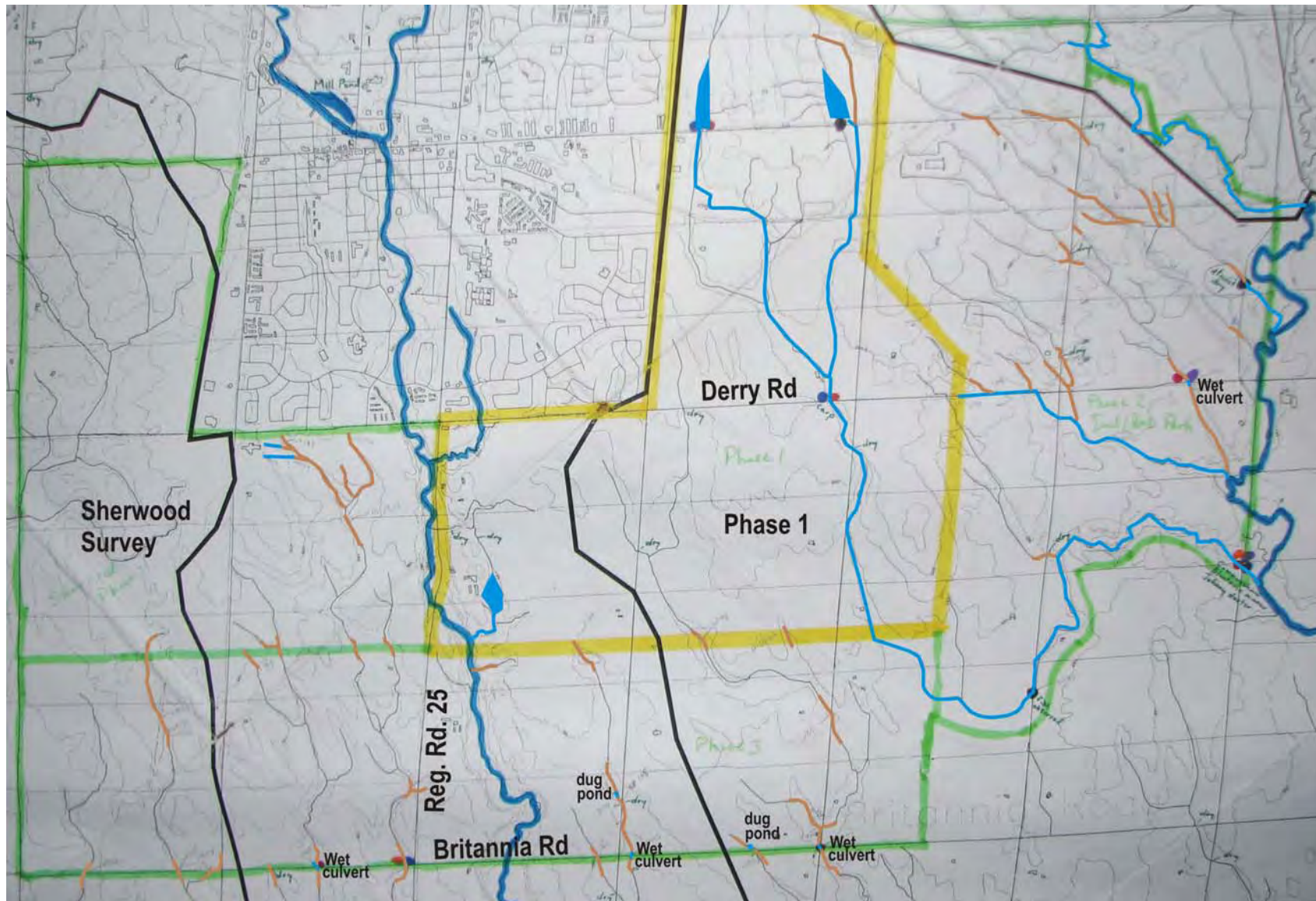
Figure 3.5.1: Reaches of watercourses that were flowing or where standing water was present (blue), or that were dry (light brown) in the autumn of 2007. The Phase 1 urban expansion lands are shown with a yellow border.
