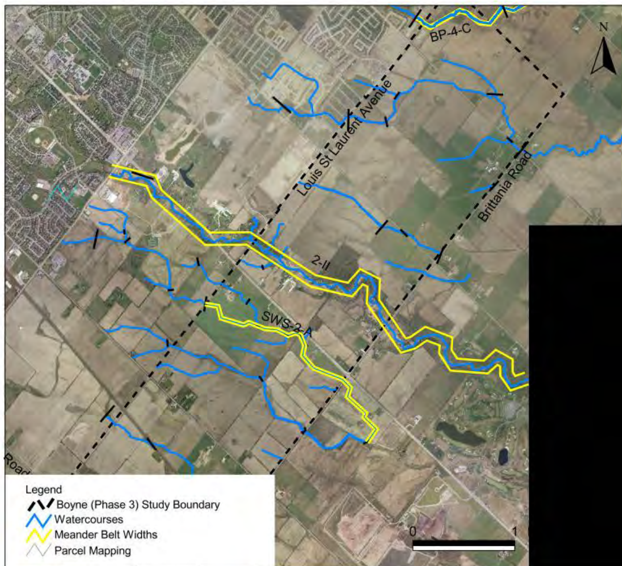
Figure 3.4.6b: Meander Belt Width delineation for the Boyne Survey (Phase 3) lands (only defined for reaches of Medium Geomorphological Constraint and above – see Section 3.4.5)
